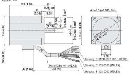
Enter the length of the connection cable (included) as 1 [1 m (3.3 ft.)], 2 [2 m (6.6 ft.)] or 3 [3 m (9.8 ft.)] in the diamond ( $\diamondsuit$ ) within the model name.
