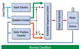
Motor runs in open loop mode like a stepping motor.
