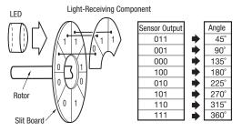
The encoder, which can detect the absolute position within a single rotation of servo motor, outputs the absolute position of rotation angle.
