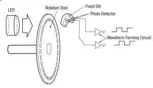
The encoder, which can detect the rotation amount, speed and direction of the servo motor, outputs the pulses depending on the alteration of rotation angle. Normally, it outputs the detected waveform without modification, so that the current position is lost during power blackouts.
