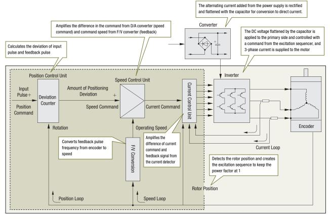
The servo motor consists of three components: a motor, an encoder and a driver. The driver compares the positioning command and position/speed information from the encoder and controls the drive current. The servo motor always detects the motor status with the positioning/speed information from the encoder.
