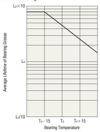
To use the motor longer, it is effective to take measures to lower the motor temperature.
