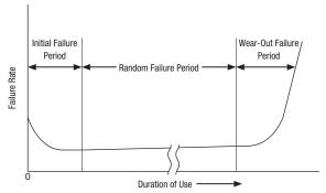
Relationship between the Duration of Use and Failure Rate
