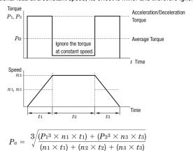
$n_1$  and  $n_3$  indicate the average number of rotations in  $t_1$  and  $t_3$  zones, respectively. In the above example, the following values apply:  $n_1 = n_3 = \frac{1}{2}n_2$
